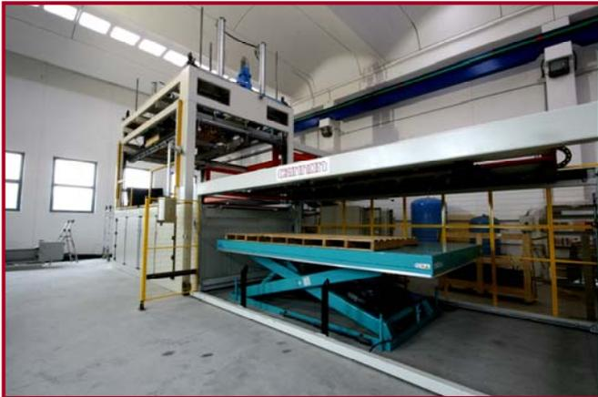
Sheet separation is less problematic because of sheet weight, but clamping the part with lifting fingers for unloading can generate issues in cases of heavy thickness HDPE and double impressions.
