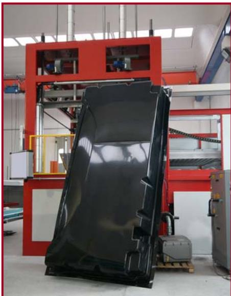
**CLAMPING SYSTEM** - Cannon improved clamp frames have toe sections to allow the heating on the edges, despite the telescopic adjustment. The clamping frame distributes the clamping pressure evenly on the perimeter of the sheet: considering that this perimeter is 13,500 mm long and exposed to serious heating this is not so trivial!
