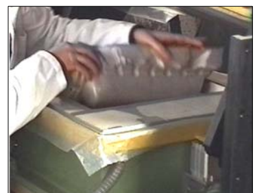
Easy release out of the mould and elimination of all cleaning and spraying operation
